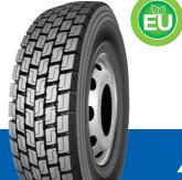
Pattern characteristic: Mixed pattern design provide strong traction and breaking power . Longer block pattern design enhance the ability of unti eccentric wear and the abnormal wear. Five deep grooves, multi blocks & tiny kerfs on the blocks assure a firm grip and a powwerful tr Suitable conditions Suitable for driving wheel position on good road condition.
